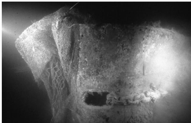
Figure 11. The bow of *AE2* enshrouded in nets. The anchor/tow chain can be seen exiting the hawse pipe, and below, out of picture is the single forward torpedo tube. Note the extensive damage caused by fouled fishing nets. Photo: Mark Spencer.
